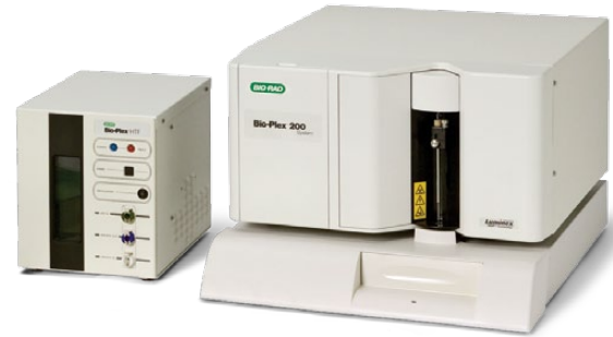
The SnapPath instrument being developed by BioMarker Strategies automates the process of preparing a live tumor sample and testing its dynamic response to multiple therapies at once. In analyzing the complex results of this process, the Bio-Plex multiplex immunoassay system proved a key solution for measuring phosphoprotein levels in pathways of interest.
